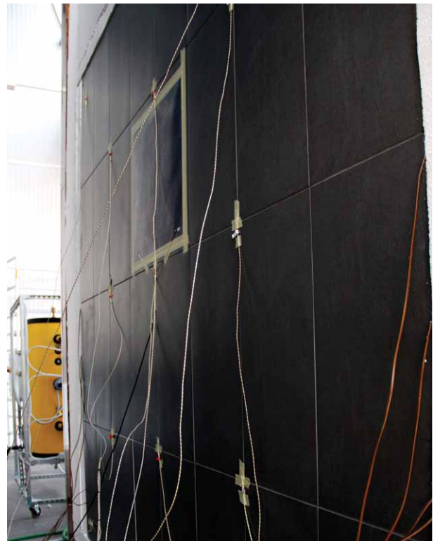
Test sample equipped with measurement sensors
