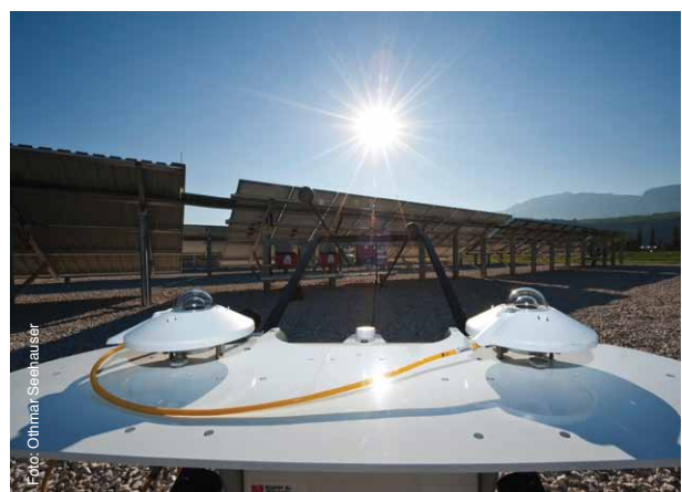
View of secondary standard (ISO 9060) pyranometers to monitor diffuse and global irradiance.
