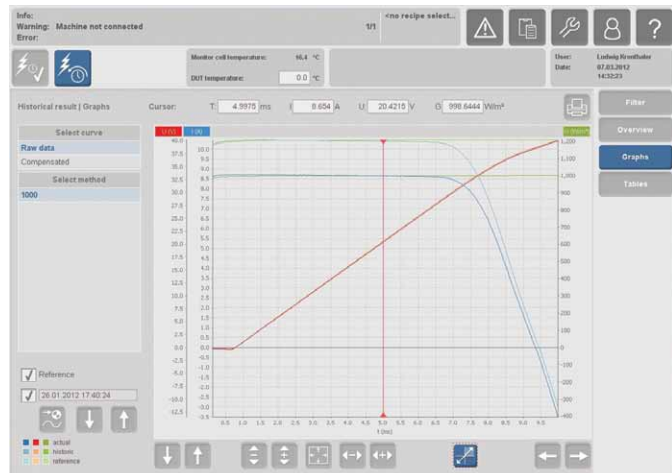
Solar simulator software: visualisation of the I-V curves
