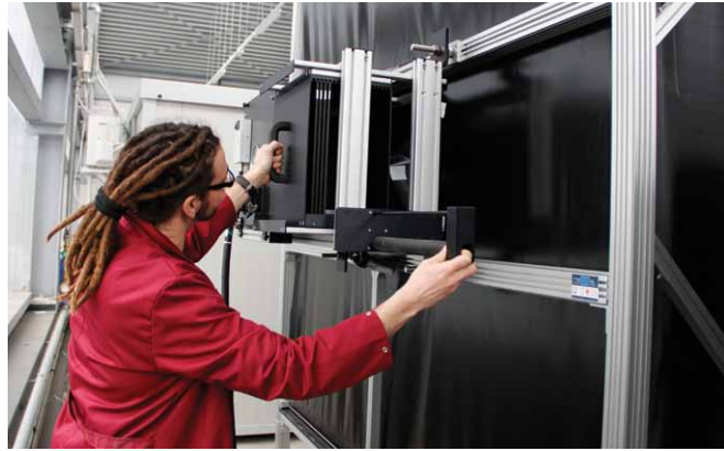
Changing the attenuation masks of the flash box at the rear of the solar simulator
