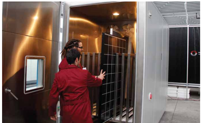
Placing the PV test modules into the climatic chamber
