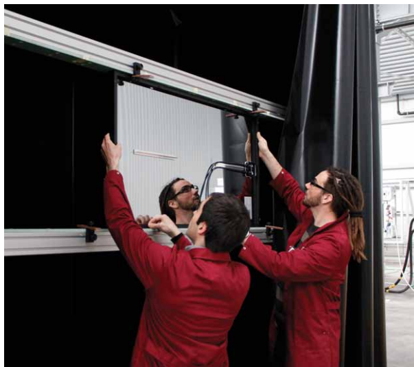
Attaching a PV module to the panel mount at the front of the solar simulator
